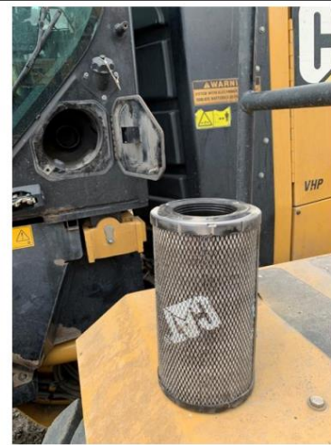
Figure 9: Grader Intake air filter – Engine grade. Not HEPA.
