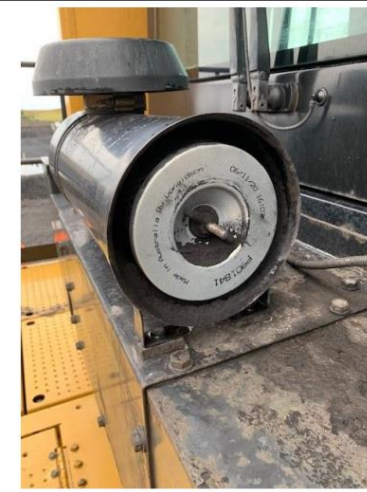
Figure 10: Cat 992K Loader Intake air filter – Engine grade. Not HEPA
