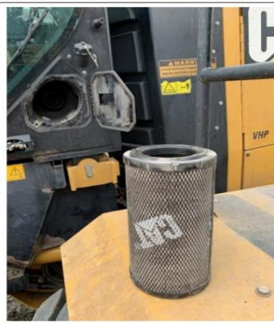
Figure 9: Grader intake air filter – Engine grade. Not HEPA.
