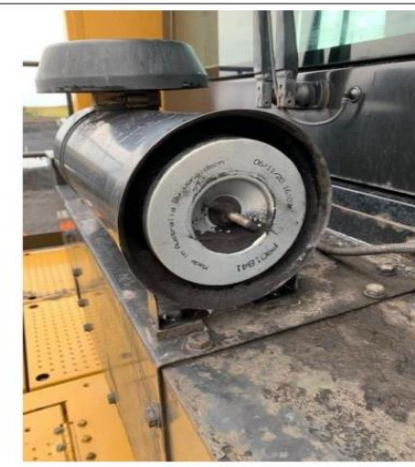
Figure 10: Cat 992K Loader Intake air filter – Engine grade. Not HEPA
