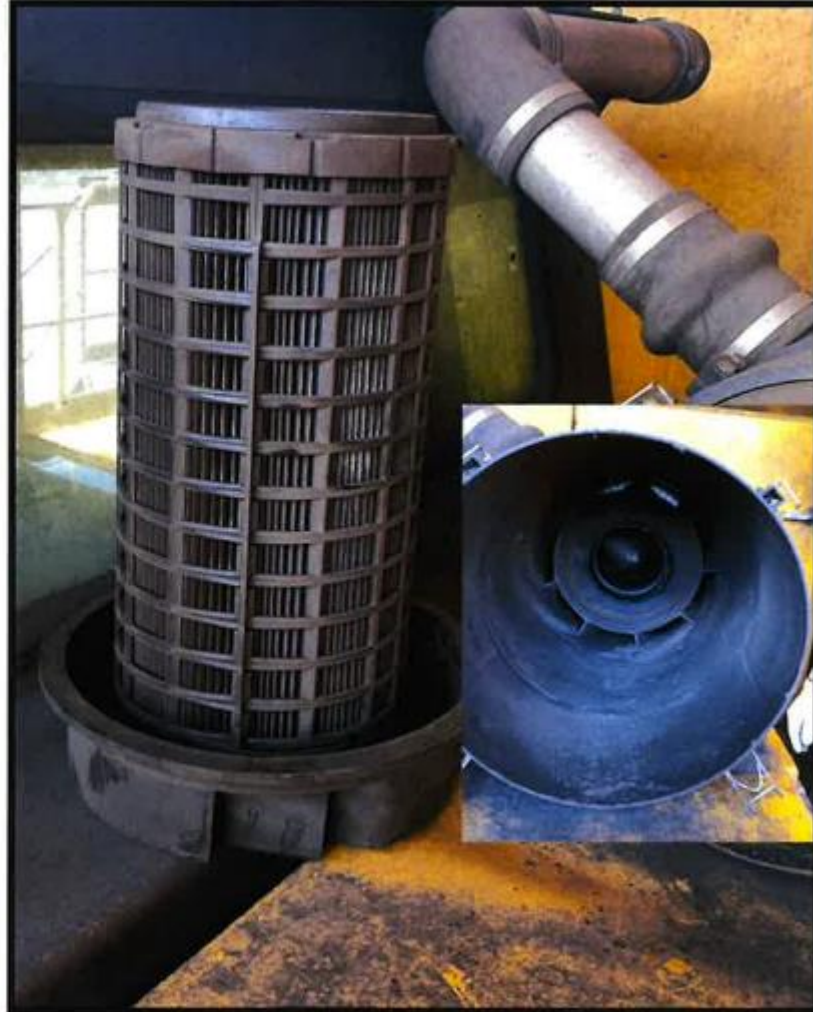
Komatsu 930E-4 ISO 23875 retrofit installation with HEPA Filter at 480 hours run time in Coal mine
